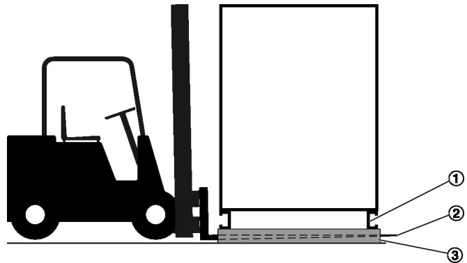
Fig. 4: Carrying load with a forklift
