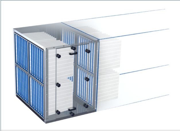
Example of variant UCA-2SPF, with pocket filters as first and second filter stages. When using pocket filters as second filter stage, the space required for the filters in the connected ductwork must be accounted for.
